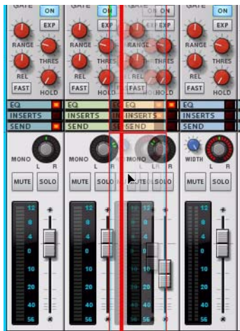
Moving a channel. The thicker red line indicates where the moved channel will be inserted.
