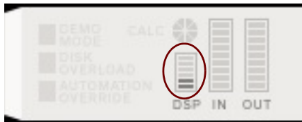
The DSP meter on the Transport Panel
