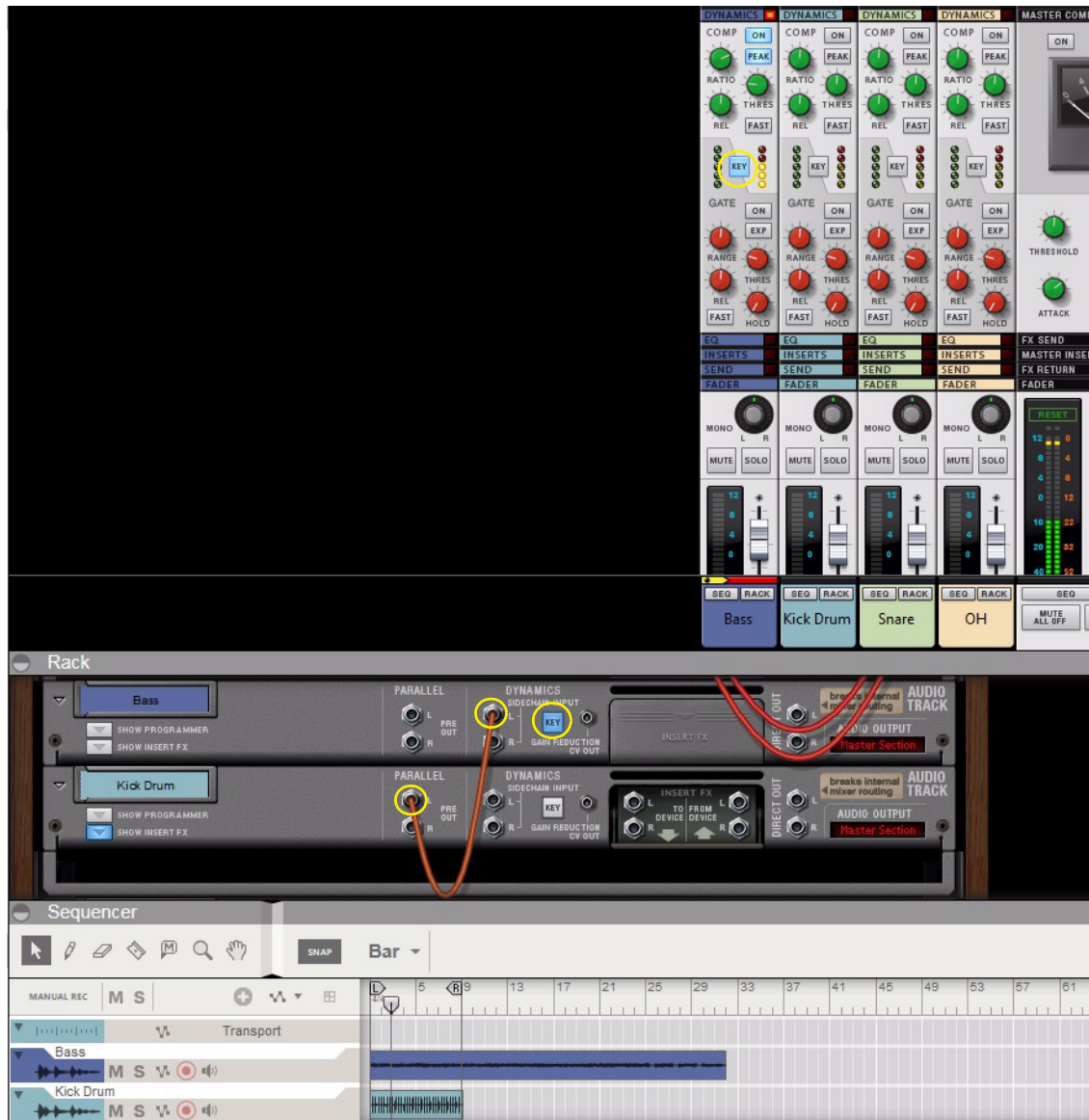
Compression Sidechaining of the Bass audio track from the Kick Drum audio track.
