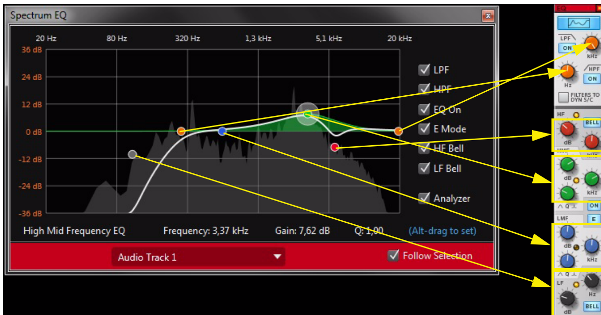
The Spectrum EQ editing objects (points) and what parameter(s) they affect in the mixer channel strip.
