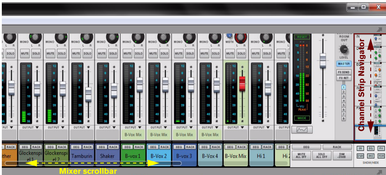
The Main Mixer with the Fader sections currently scrolled into view.
